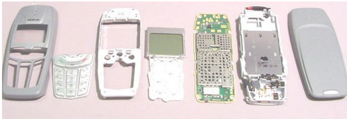
The main parts of the phone disassembled.
